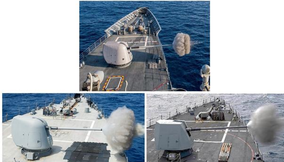
Figure 3.0-2: Gun Blast and Projectile from a MK 45 MOD 2 5-inch/54 Caliber Navy Gun on a Cruiser (top), a MK 45 MOD 2 5-inch/54 Caliber Navy Gun on a Destroyer (bottom left), and a MK 45 MOD 4 5-inch/62 Caliber Navy Gun on a Destroyer (bottom right)
