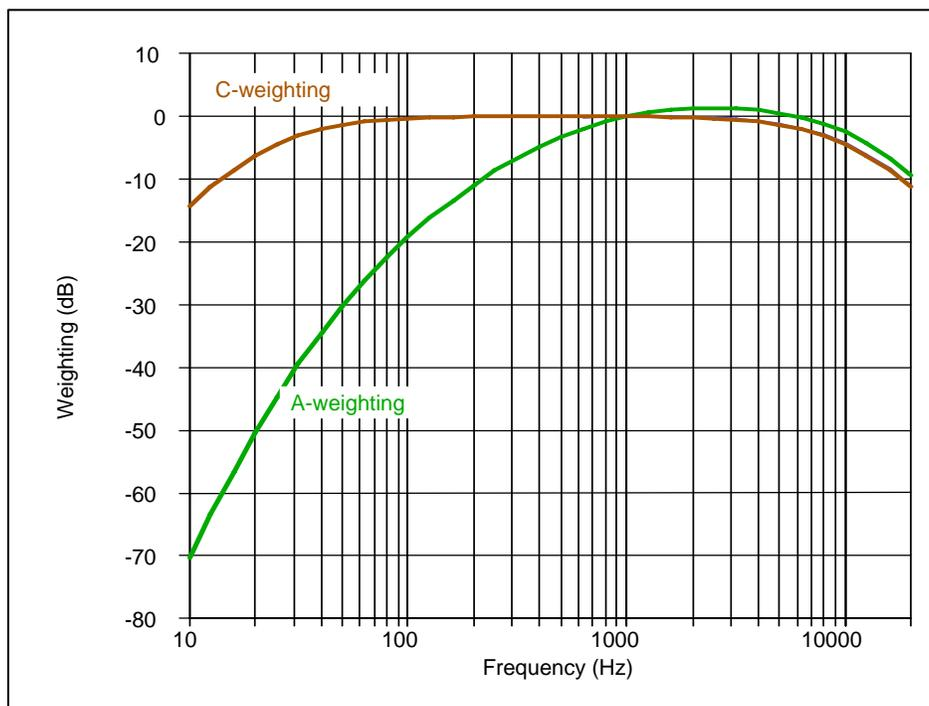
Figure E.1-4 Frequency Responses for Sound Level Weighting Characteristics
