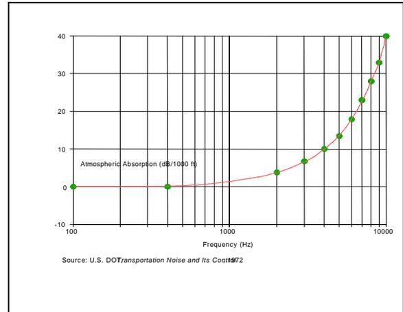
Figure E.1–1 Typical Effect of Frequency on Atmospheric Absorption of Sound
